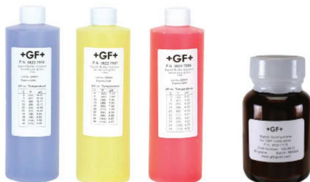
All pH buffers are color coded for easy identification; 4.01 pH is red, 7.00 pH is yellow, and 10.00 pH is blue. All pH buffers are traceable to NIST standards. The 4.01 and 7.00 pH buffer solutions can be used to calibrate ORP sensors when saturated with quinhydrone.
