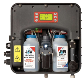
CLX Instrument cover removed
